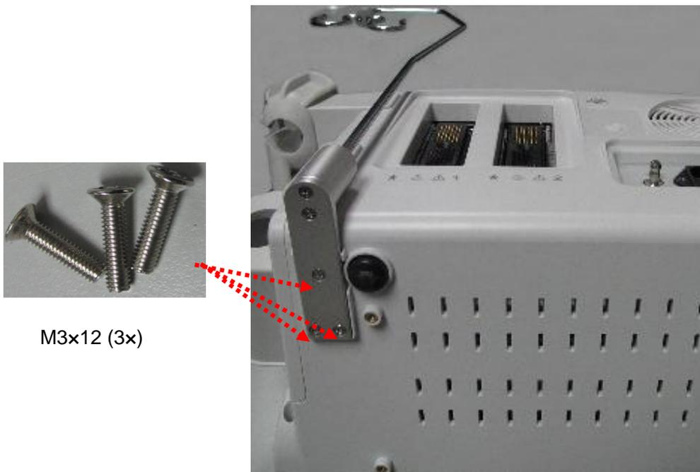
Figure 4-1 Assembling Cable Holder to Main Unit
