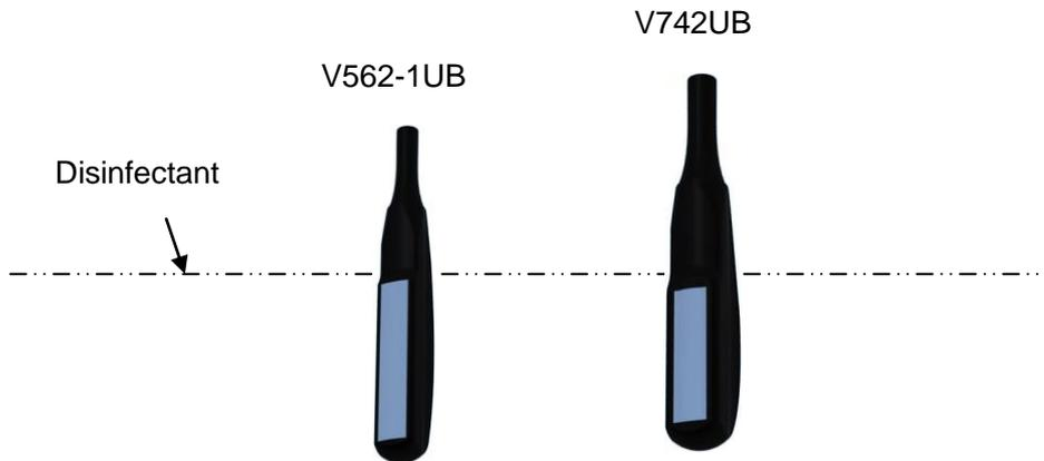
Figure 12-1 Depth of the Transducer Immersed into Disinfectant
