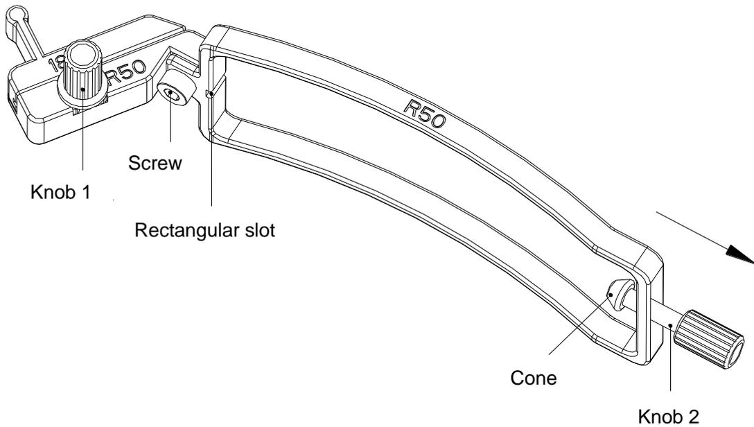
Figure 6-28 Structure of Needle Guide Bracket Kit
