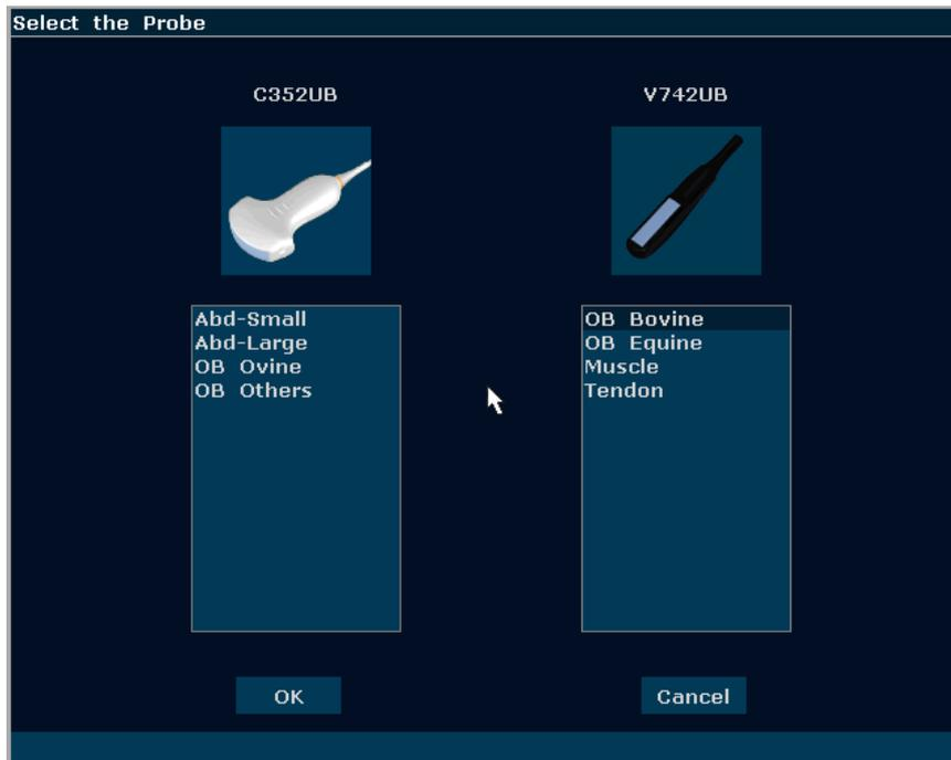
Figure 6-2 Probe and Examination Selection Menu
