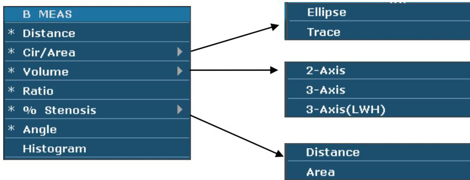
Figure 6-3 B Mode Generic Measurement and Calculation Menu
