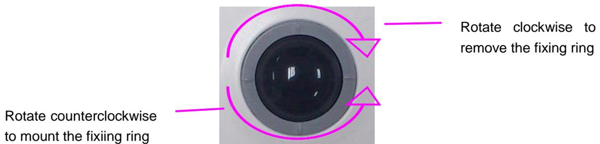
Figure 12-2 Assembling and Disassembling Trackball
