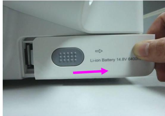
② Pull the battery compartment door out
