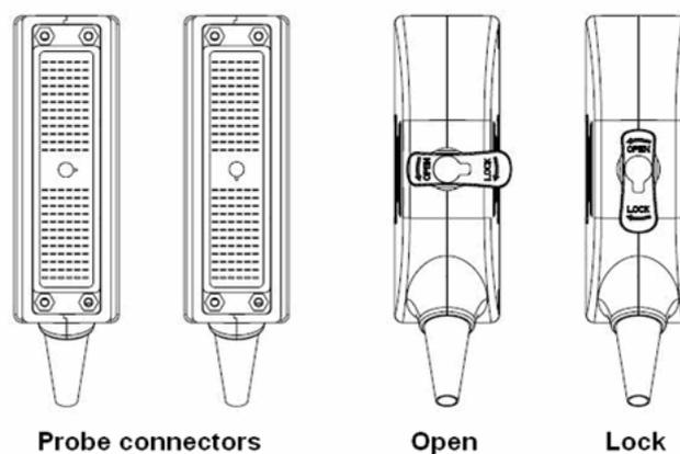
Figure 4-6 Lock and Open Marks on Probe Connectors
