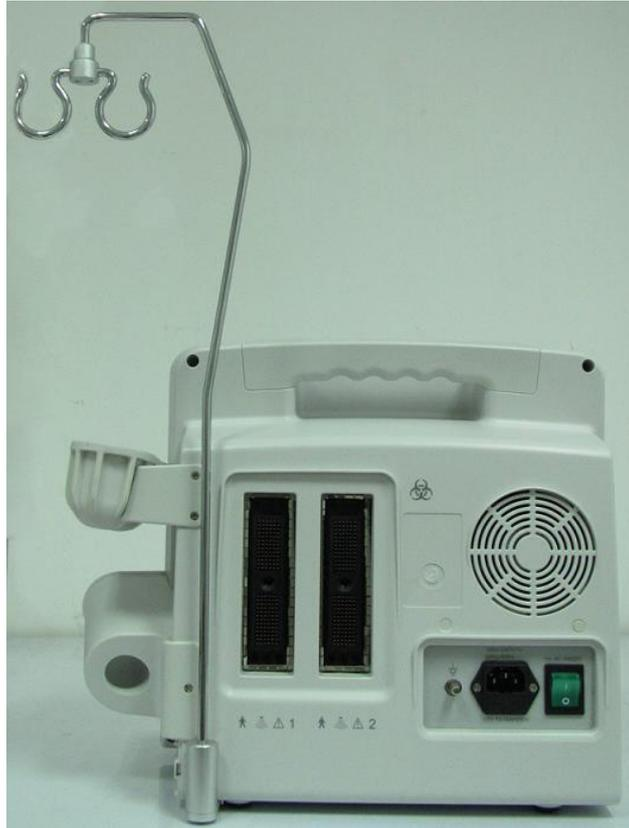
Figure 4-2 Main Unit with Cable Holder
