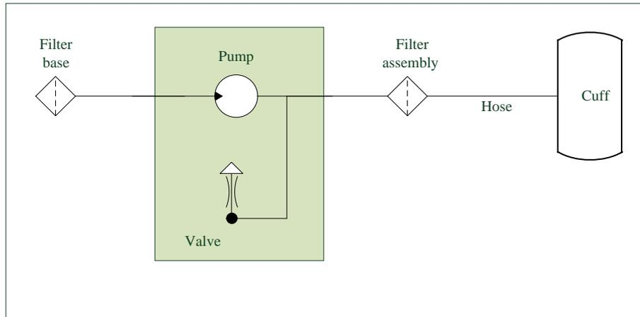
The recommended cleaning frequency is once every month, if the environment is dusty, the frequency may be twice every month, if the sound during inflation is noisier than usual, user needs to clean the dust-proof filter assembly according to the real condition.
