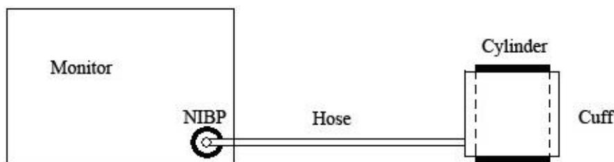
Figure 4-1 Diagram of NIBP Air Leakage Test
