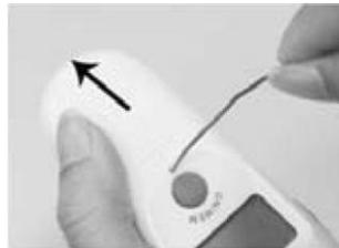
2. Hold the thermometer and flip the battery out with a small screwdriver.
