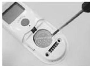
3. Insert the new battery under the metal hook on the left side ① and press the right side ② of the battery down until the it clicks in place.
