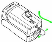
Figure 4 Installation de corde
