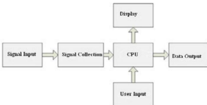
Figure 7-1 System Principle
