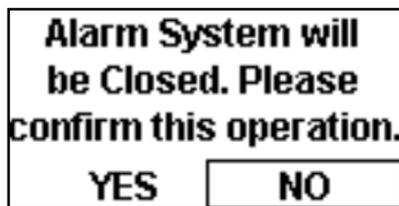
Figure 3-12 Confirm to Turn off Alarm
