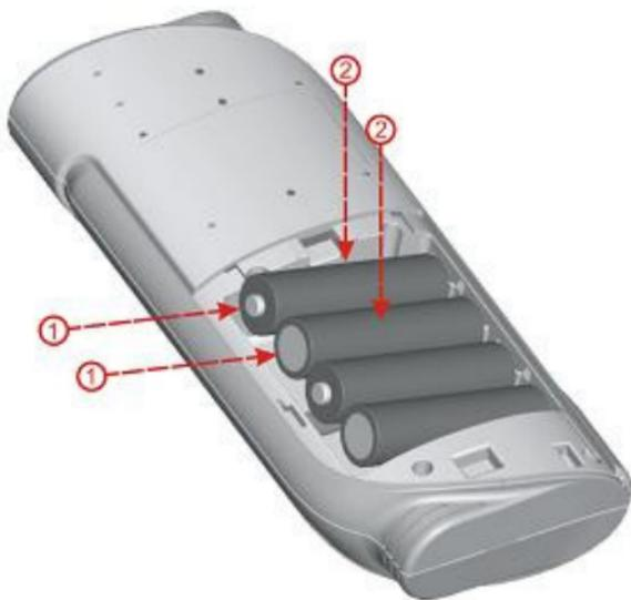
To install the rechargeable Ni-MH battery package:
