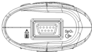
Figure 2-6 Sensor and Cable Connecting Port
